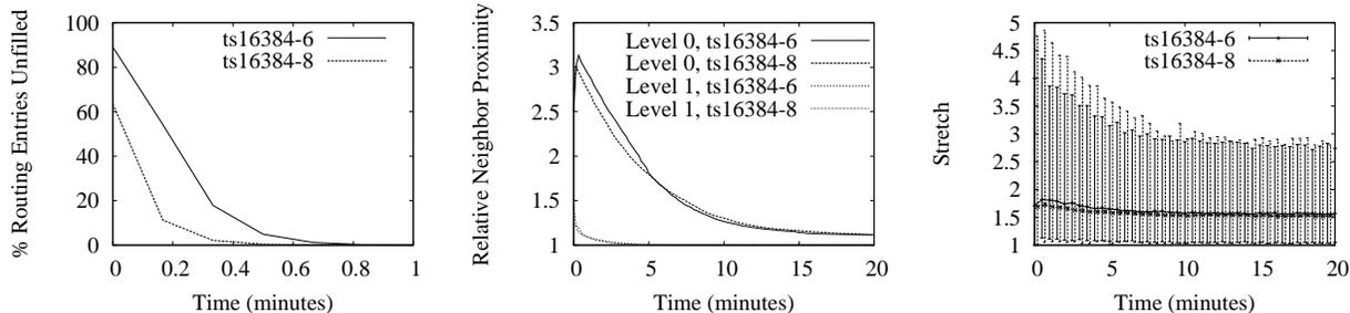
Figure 14: *Bamboo performance in a static network.* From left to right, shown are the percentage of fillable routing table entries that are unfilled, the mean relative proximity of those entries compared to optimal, and the resulting stretch observed for routes through the DHT. Note that the leftmost graph has a different time scale.
