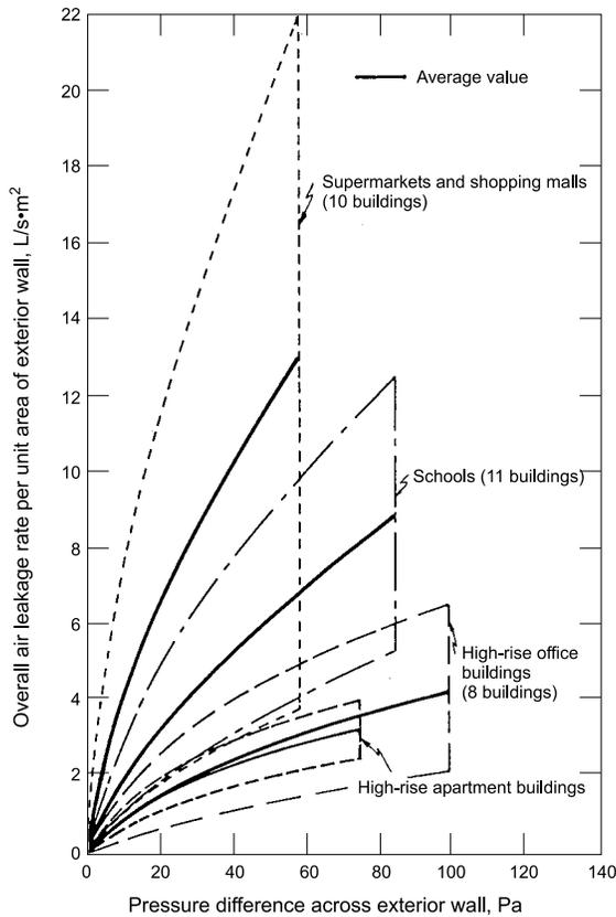
Figure 3. Airtightness measurements in various types of buildings
