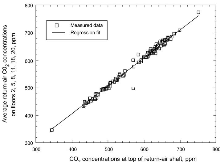
**Figure 8.** Comparison of CO<sub>2</sub> concentrations measured at the top of the return-air shafts and at return-air intakes on individual test floors
