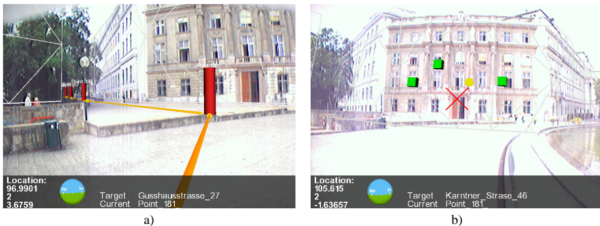
Fig. 2. a) The navigation application shows the way points and connecting paths to the user. b) A user can set annotation icons by controlling a ray cast into the scene. Both images are screen shots of the mobile setup in video see-through mode.
