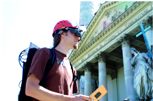
Fig. 1. A mobile user roaming historical locations in the city of Vienna. He is equipped with a see-through HMD, a video camera, inertial tracker and GPS receiver mounted to a helmet. The mobile AR system is mounted to a backpack.
