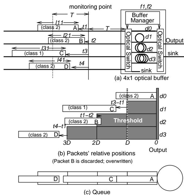
Figure 4. Behavior of packets arriving at the optical buffer (vPBSO)
