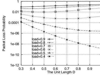
Figure 3. Performance dependence on  $D$  (unit delay normalized by mean packet length). The number of fiber delay lines  $B = 50$ .
