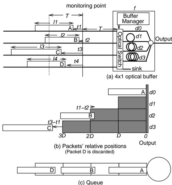
Figure 2. Fundamental behavior of packets arriving at the optical buffer
