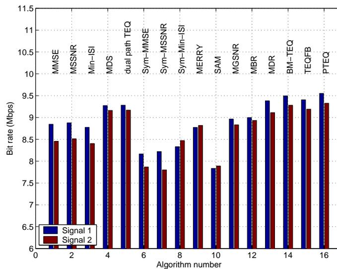
Fig. 6. Bit rate achieved using the two measured AST channels. The channel impulse responses are given in Fig. 5.
