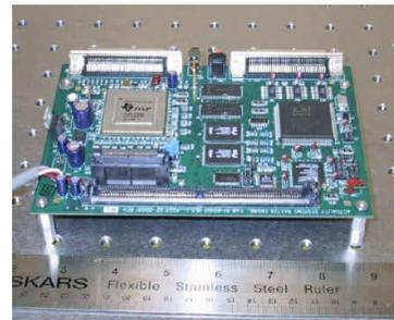
Fig. 4. Photograph of raster engine, which converts 3-D image data into a time-sequence of 2-D "image slices."
