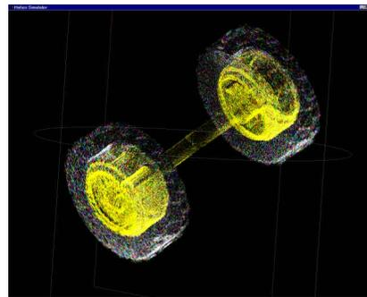
Fig. 8. Screenshot of the 3-D display simulator, which simulates the swept-screen architecture, rasterization, and simulated hidden-surface removal algorithms.
