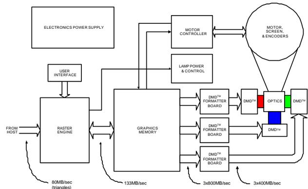
Fig. 3. System electronics.
