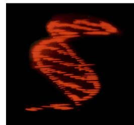
Fig. 1. Photograph of  $64 \times 64 \times 64$  multiplanar display as described in [9].
