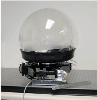
Fig. 5. Photograph of the projection system and screen inside rotating dome.
