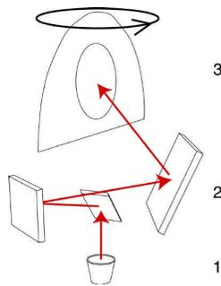
Fig. 2. Schematic illustration of 3-D display principle. A fast projector (1) illuminates a rotating projection surface (3) via several relay mirrors (2) which rotate with the screen. The projector and control electronics are fixed.
