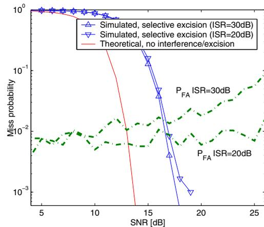
**Fig. 5.** Chirp interference and domain selective interference excision, ISR is 20 dB or 30 dB and the bandwidth swept during the detection interval is 100 % of the system bandwidth.
