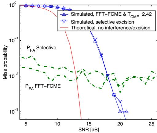
**Fig. 3.** Sinusoidal interference, frequency domain and domain selective interference excision, ISR is 20 dB per sinusoidal signal and the number of sinusoidal signals is 2.
