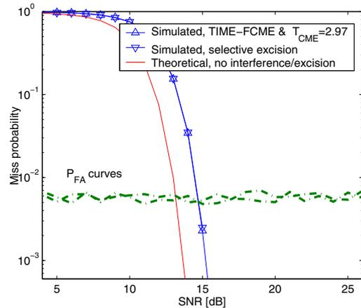
**Fig. 4.** Impulse interference, time domain and domain selective interference excision, ISR is 30 dB and 40 % contamination.
