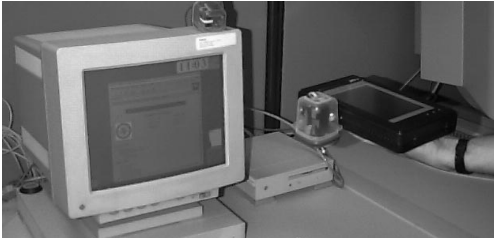
Figure 7. Home-made IR units allow cross-platform communication.
