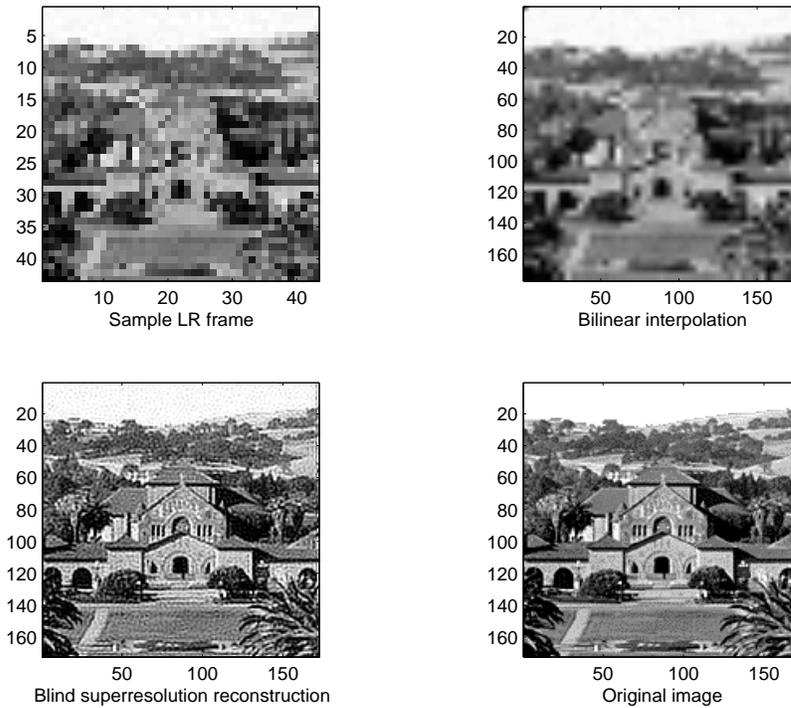
Figure 4: Blind superresolution for synthetic sequence - example I, 30dB.
