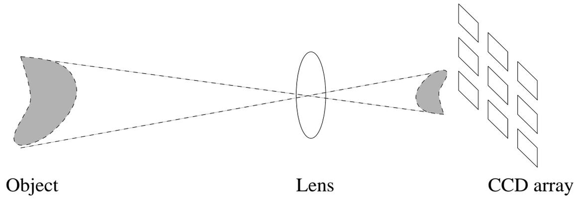
Figure 2: CCD camera model.
