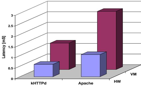
Figure 6: Latency effects of commercial VM technology (VMware 3.2.0)
