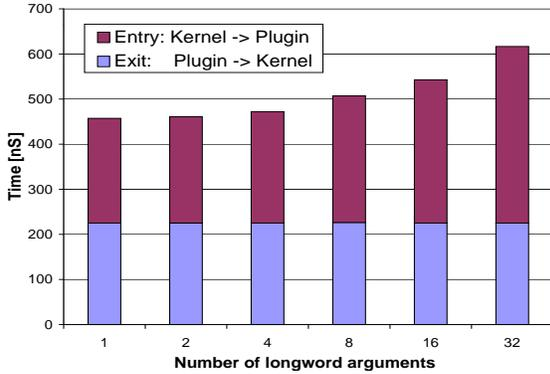
Figure 5: Control transfer cost vs. number of arguments
