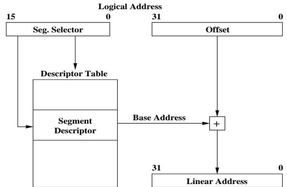
Figure 3: Intel x86: logical to linear address translation
