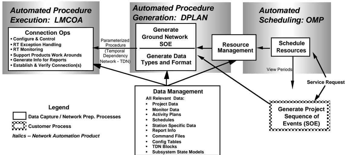
**Figure 1: Automation technology applied to DSN operations processes**
