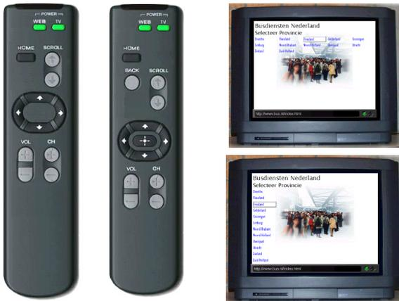
Figure 2: (left) linear-oriented remote control; (middle) plane-oriented remote control; (right upper corner) matrix layout; (right lower corner) list layout.
