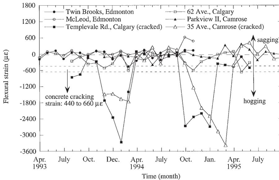
Fig. 13. Comparison of normalized flexural strains with time.
