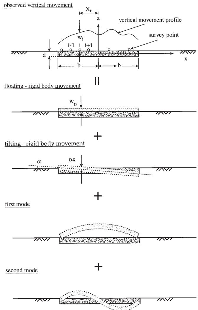
measurement errors. Four possible methods, finite difference, cubic spline, polynomial fit, and Fourier series methods, were examined to obtain estimates of flexural strains (Zhan and Rajani 1995). The Fourier series method with one sine term was identified as the most suitable method. Histories of rigid body movements and flexural strains are determined to assess their association with changes in climatic conditions.
