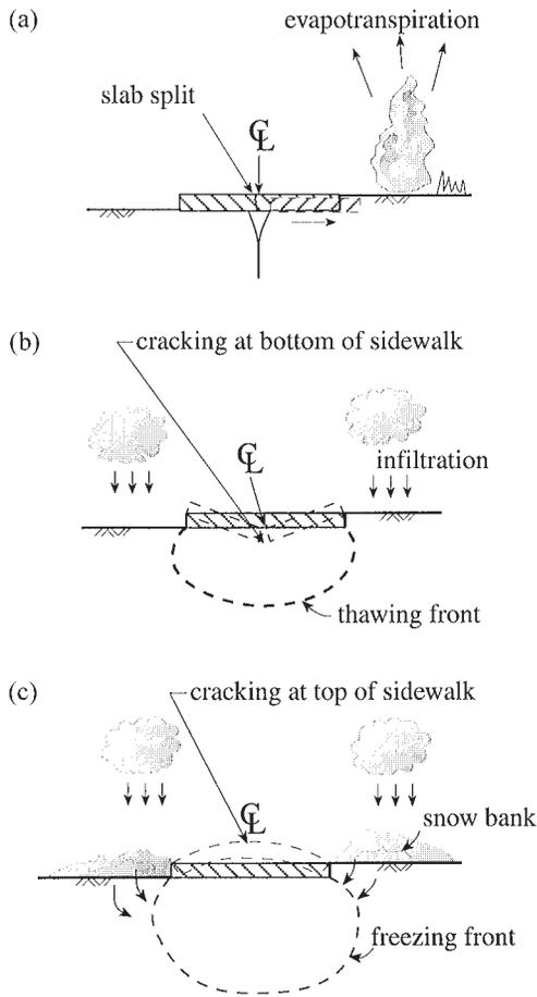
**Fig. 8.** Components of vertical movement for a typical sidewalk slab.
