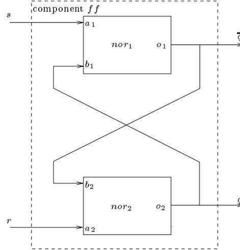
Figure 7.2: RS-flip-flop example
