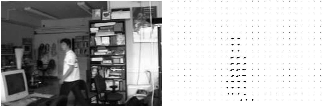
Figure 5: Optical flow results for the Lab image pair.
