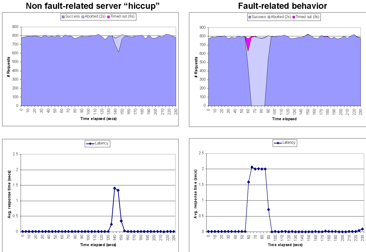
Figure 9: A comparison of the throughput components and latencies of an HA-PRESS system during a spontaneous “hiccup” caused by resource exhaustion and an actual fault. Note that the response times reach the connection abort time limit of two seconds during the actual failure, resulting in a 30-second interval during which all client requests either abort or time out. The service disruption that the spontaneous “hiccup” causes is comparatively minor.
