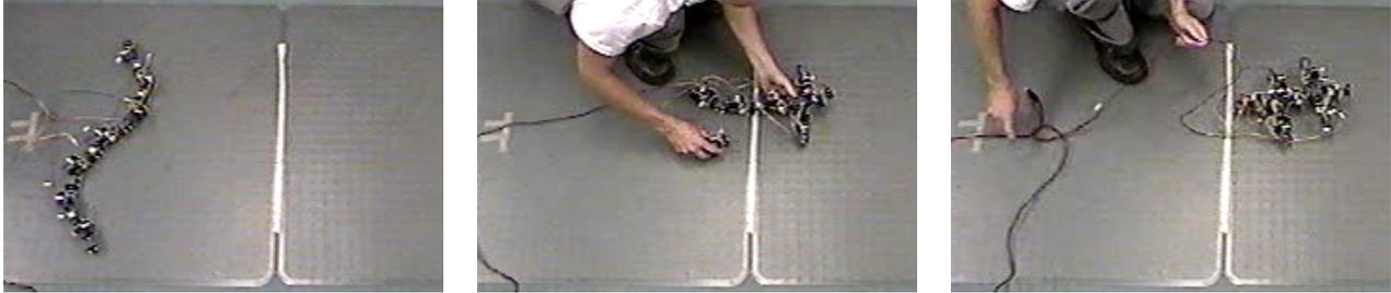
Figure 5: The robot first covers a distance of 63cm configured as a sidewinder (left). The robot is then manually reconfigured into a quadruped walker (middle). Finally the robot walks 87cm (right). Note that the cables only provide power.
