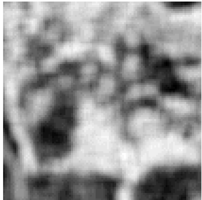
Fig. 2. Mean Entropy feature map for the area shown in figure 1. Lighter shades mean greater entropy.
