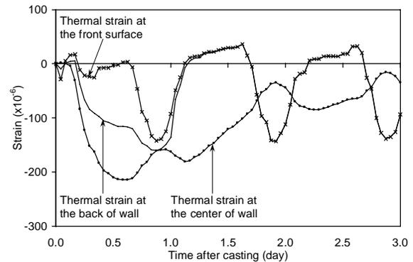
Fig. 8 – Estimated thermal strains in barrier wall at midheight
