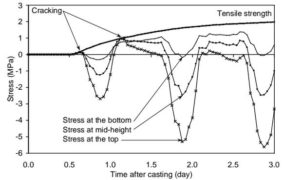
Fig. 11 – Estimated total stress at front surface of barrier wall near midspan
