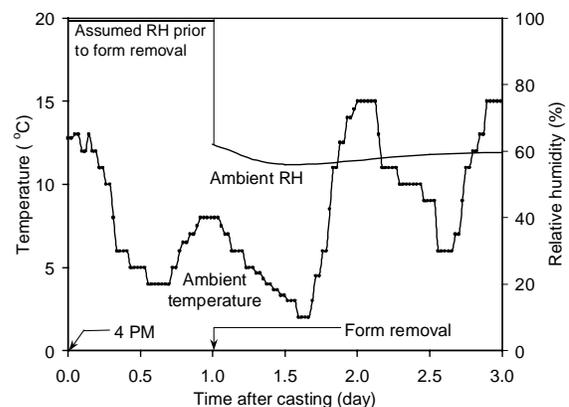
*Fig. 2 – Measured ambient temperature and ambient relative humidity*
