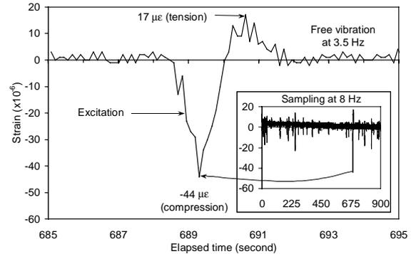
**Fig. 10 – Estimated traffic-induced strain at top of barrier wall at midspan**
