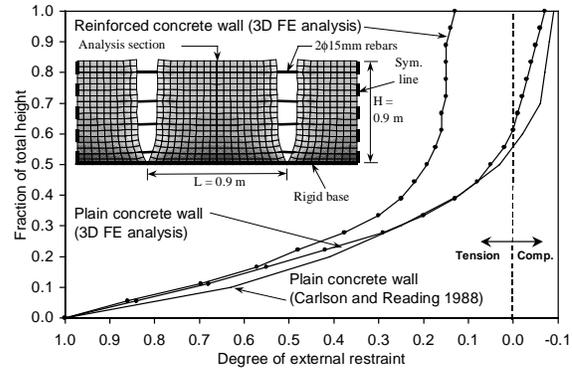
Fig. 5 – Estimated external restraint in plain and reinforced concrete walls with  $L/H=1$  (elevation view of the wall model)
