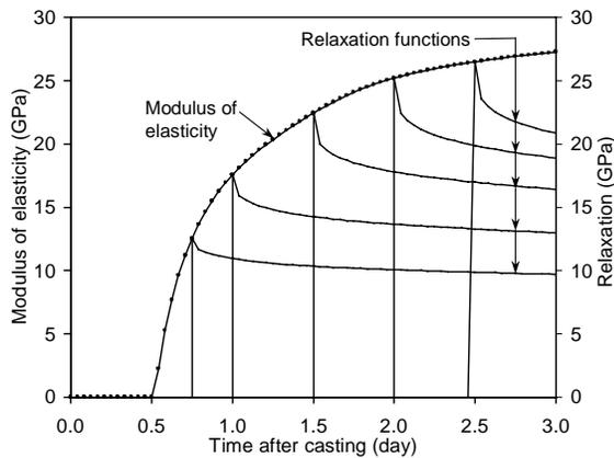
Fig. 4 – Estimated modulus of elasticity and relaxation functions of barrier wall concrete
