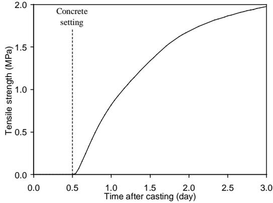
Fig. 3 – Estimated tensile strength of barrier wall concrete
