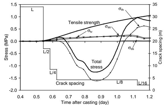
Fig. 12 – Estimated stress components in barrier wall (front surface, midheight, midspan)
