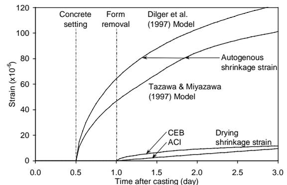
Fig. 9 – Estimated shrinkage strains in barrier wall
