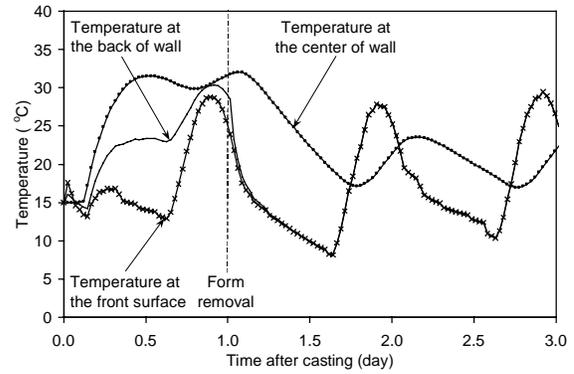
**Fig. 7 – Estimated temperature variations in barrier wall at midheight**
