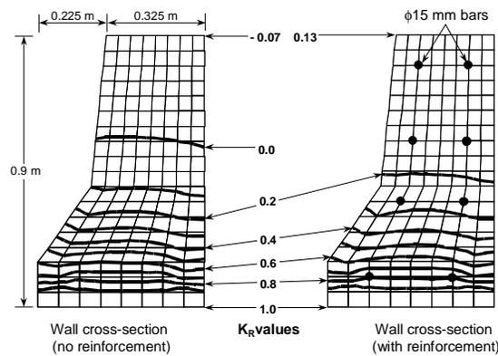
Fig. 6 – Estimated external restraint in plain and reinforced concrete walls with  $L/H=1$  (cross section view of the wall model)
