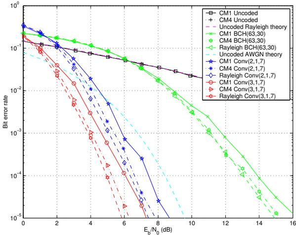
Fig. 4. The bit error rate of an uncoded system and with convolutional codes (2,1,7) and (3,1,7) and the BCH(63,30) code on IEEE channel models CM1 and CM4 without shadowing and uncorrelated Rayleigh fading.
