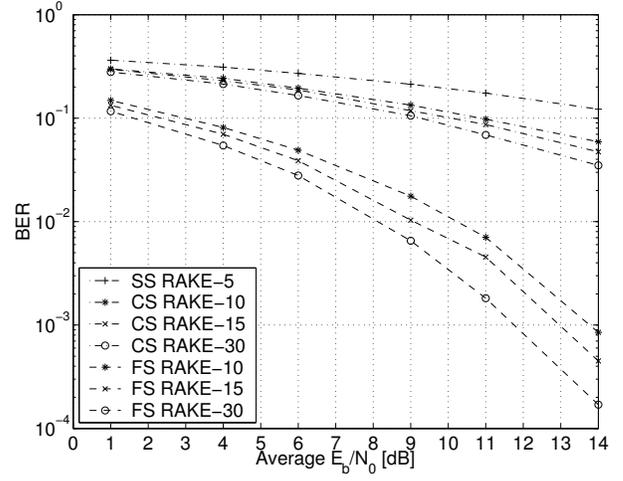
Fig. 1. The bit error rate of symbol-, chip-, and fractionally spaced Rake receivers with perfect channel estimation for DS-UWB on CM1 with shadowing.
