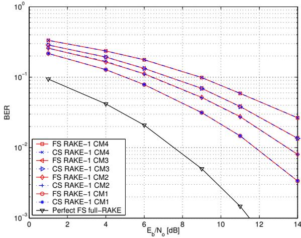
Fig. 3. The bit error rate of chip- and fractionally spaced Rake receivers with 1 finger and sliding window.
