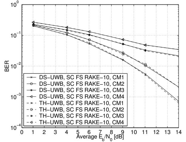
Fig. 2. The bit error rate of TH-UWB and DS-UWB with fractionally spaced Rake receivers using the successive cancellation algorithm and  $N_p = 100$  pilot bits on CM1–CM4 with shadowing.
