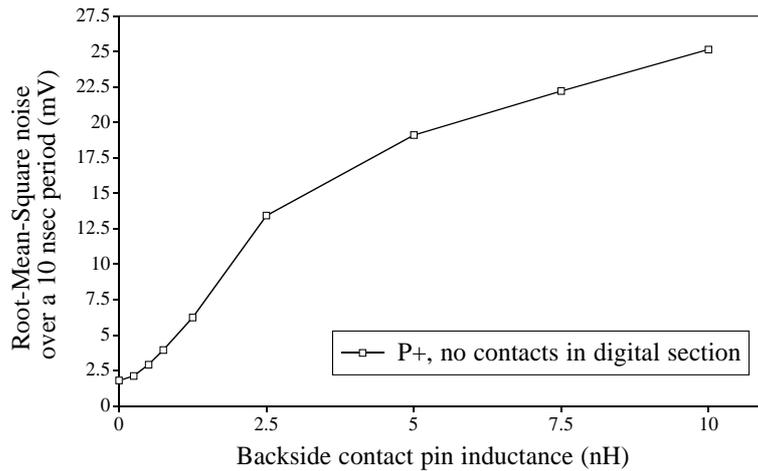
Figure 5.- Noise dependence on backside contact pin inductance. Under a certain limit, bounce in the P+ region is drastically minimised.
