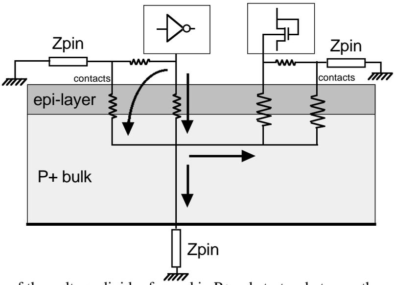
Figure 4.- Schema of the voltage divider formed in P+ substrates, between the resistance through the epi-layer, and the impedance of the backside contact pin.
