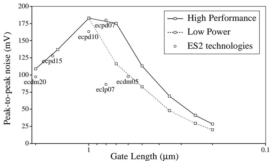
Figure 6.- Predicted trends for substrate noise in future technologies, lightly doped substrates.
