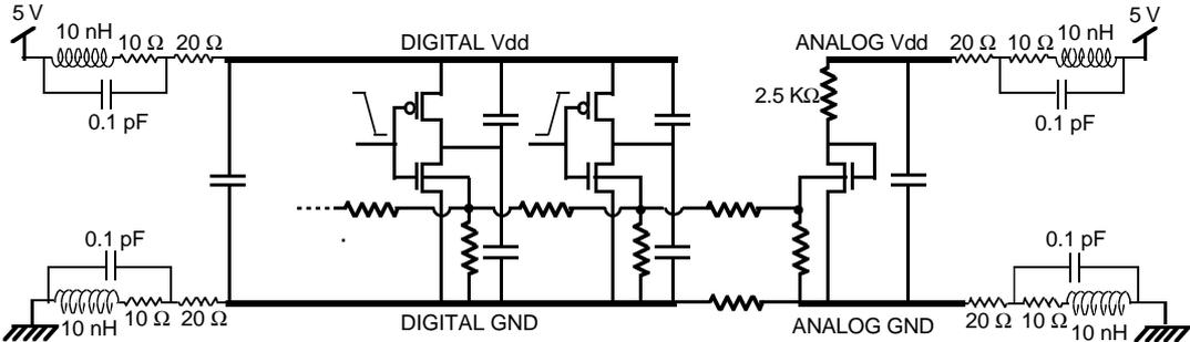
Figure 2.- Diagram of the situation analysed, including parasitic elements for the substrate and package pins, lightly doped substrate biased by the digital (left) and analog (right) ground lines.
