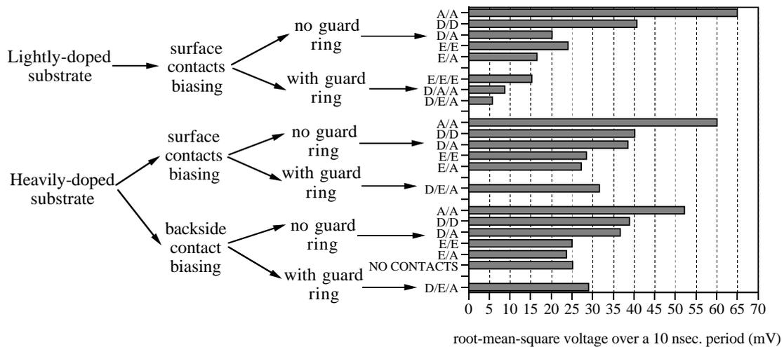
Figure 3.- Comparison of the noise coupled in function of the different biasing approaches and substrate type.
