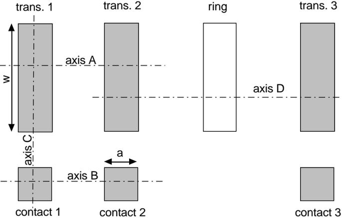
Figure 1.- To extract resistances between pairs of elements, two dimensional simulations are done along vertical sections of the layout.
