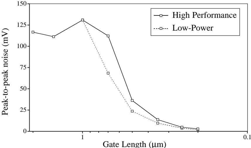
Figure 8.- Predicted trends for substrate noise in future technologies, highly doped substrates.
