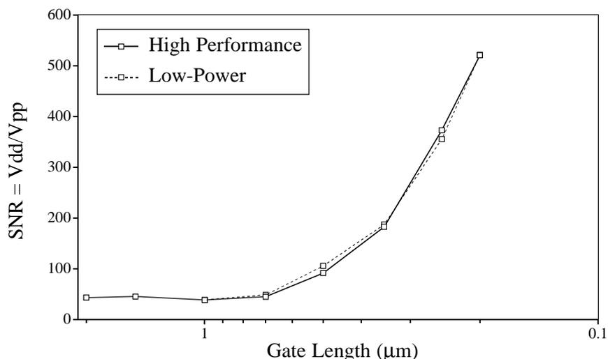
Figure 9.- Expected evolution of signal degradation due to substrate coupling.
