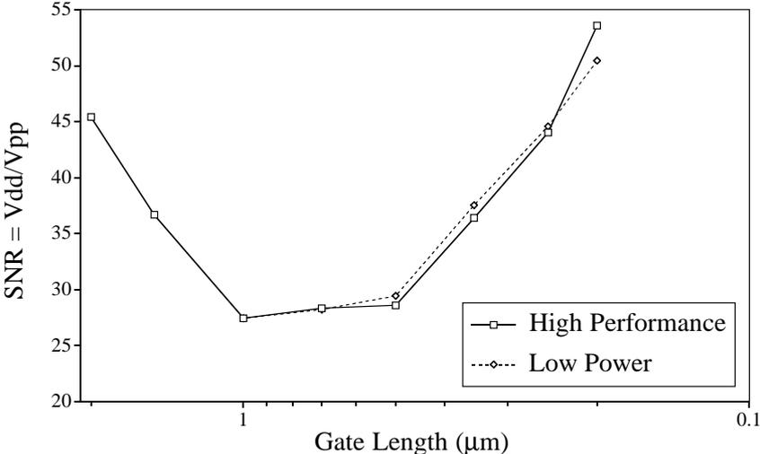
Figure 7.- Expected evolution of signal degradation due to substrate coupling.
