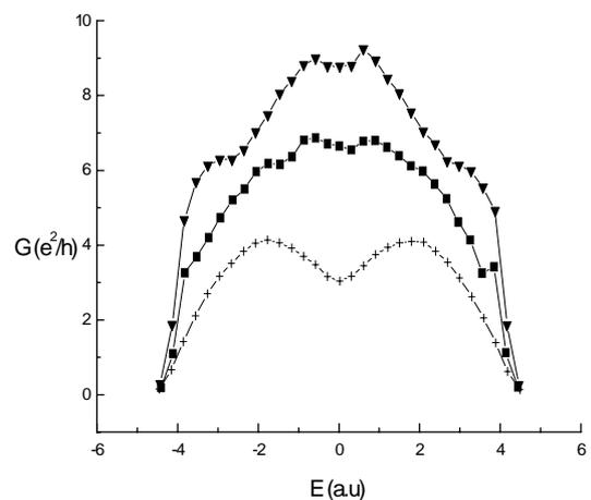
Figure(4): The averaged electrical conductance versus energy for a 35X35 substitutionally disordered binary alloy in the absence and the presence of the uniform and the random magnetic field. ( $\blacktriangledown$ ) Uniform magnetic field; ( $\blacksquare$ ) Random magnetic field, (+) Zero magnetic field.
