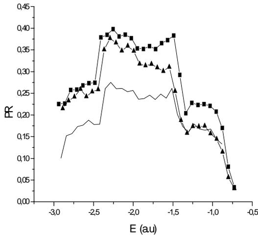
Figure(6): The averaged participation ratio versus energy in an amorphous binary alloy with 500 atoms in the absence and the presence of the uniform and the random magnetic field. ( $\blacktriangle$ ) Uniform magnetic field; ( $\blacksquare$ ) Random magnetic field, ( $—$ ) Zero magnetic field.
