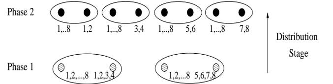
**Figure 5: Example of the hierarchical distribution stage for  $N = 8$  and  $i = 2$**
