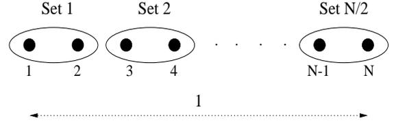
**Figure 3: Example of a sensor network with cooperation set size  $i = 2$**
