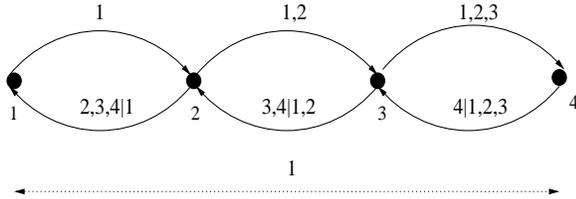
**Figure 2: Forward/Reverse cooperation over a 4 node sensor network**
