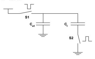
Figure 3. A Switched-capacitor "RC" circuit with S2 moved to the bottom plate.
