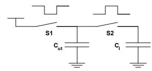
Figure 2. A Switched-capacitor "RC" circuit.
