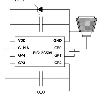
Figure 8. The iGlassware glass schematic.
