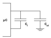
Figure 4. The microcontroller-based capacitance measurement circuit.
