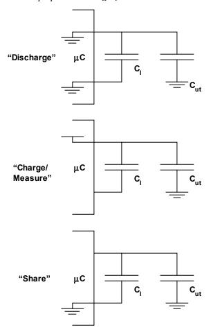
Figure 5. I/O sequence for capacitance measurement. "Charge/Measure" and "Share" are repeated until the input reads low during "Chrage/Measure". Note that the I/O pins should be set to input between steps.
