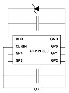
Figure 6. Ignatov's PIC-based RFID tag [6].
