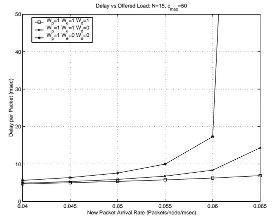
Fig. 4. Average delay per packet for different routing metric coefficients
