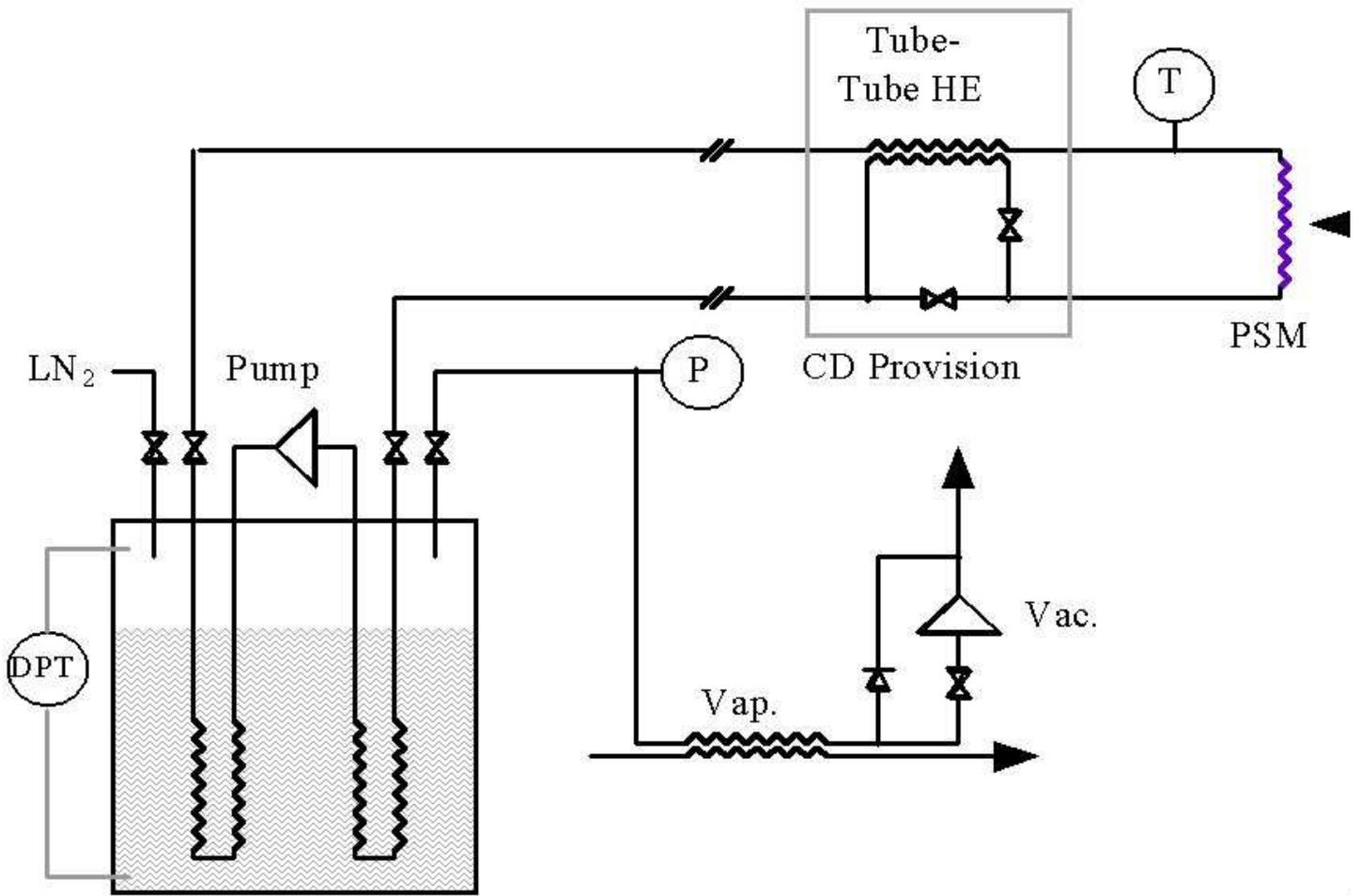
Figure 7: Scheme of cooling of the 15-T pulsed magnet via flow of He gas that is passed through a LN<sub>2</sub> heat exchanger [8].
