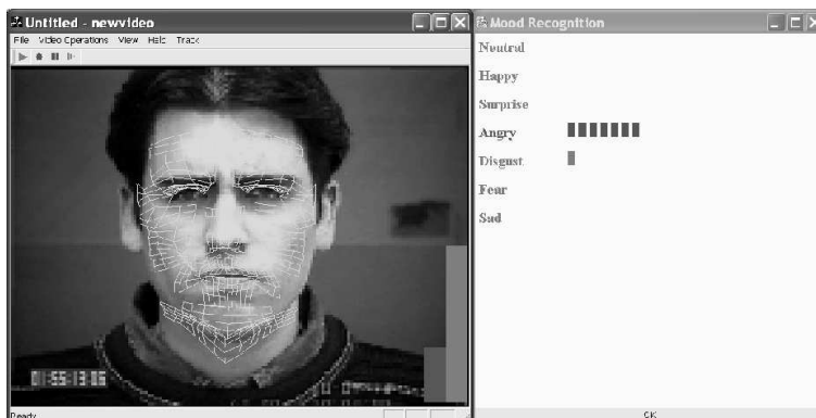
Fig. 6. A snap shot of our realtime facial expression recognition system. On the right side is a wireframe model overlaid on a face being tracked. On the left side the correct expression, Angry, is detected (the bars show the relative probability of Angry compared to the other expressions).
