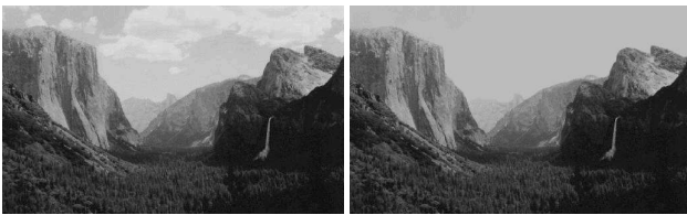
Figure 4: An example of varying the number of gray levels in image segmentation. Top: the segmented image using 72 gray levels. Bottom: the segmented image using 48 gray levels. Note that the clouds have faded into the sky in the 48 gray level image.
