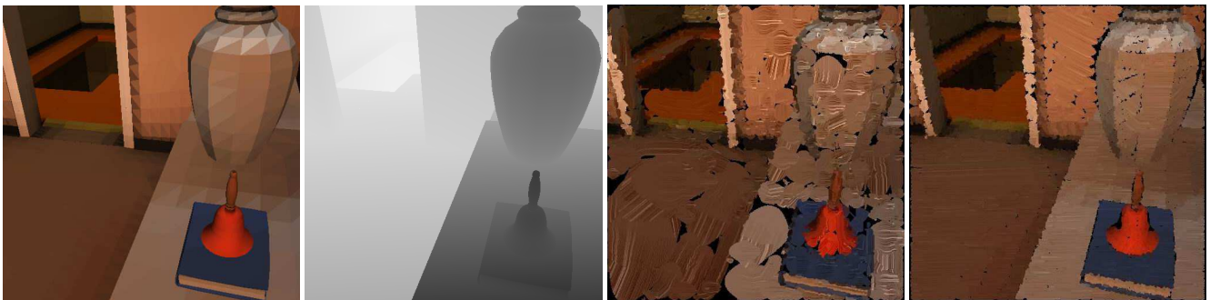
Figure 16: An example of using depth segmentation. From left to right: the original image, the depth image, the painting without using the depth information, and the painting using depth information. No underpainting was used (for comparison)
