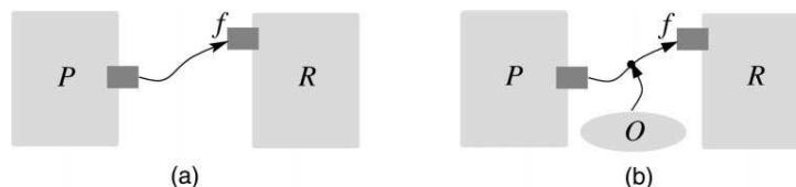
Fig. 1. Method invocation semantics. (a) Default method invocation semantics. (b) Security constraints on method invocations.
