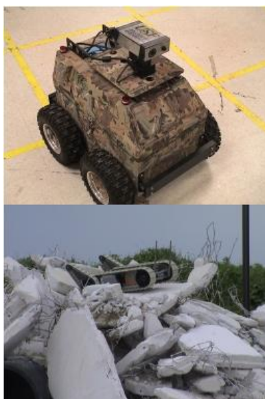
Fig. 3. A man-portable general purpose field robot (top), and a MOUT field robot exploring a rubble pile (bottom), all from manufacturer Field Y.
