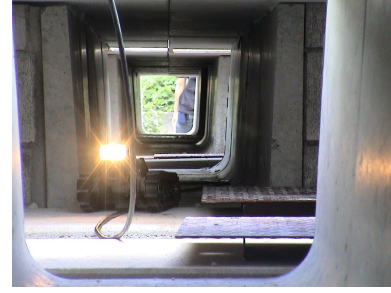
Fig. 2. Field X man-packable inspection robot in a confined space.
