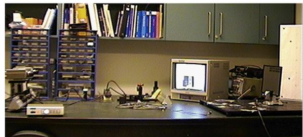
Figure 4: Experimental setup. The stereo camera pair (on the left) views a mirror and calibration target (on the right). A visual target is mounted between the two video cameras.
