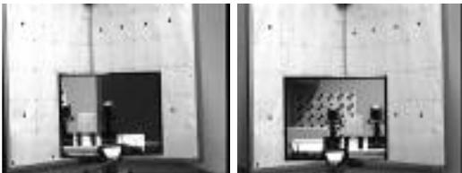
Figure 5: Stereo pair of a mirror. The reflection of the target mounted between the two cameras is clearly visible.
