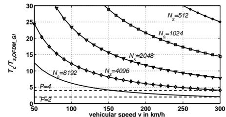
Fig. 9.  $T_{c,1}/T_{s,OFDM\_GI}$  for vehicular speed  $v$ ,  $f_0 = 5\text{GHz}$ ,  $T_{s,SC} = 7.4n_s$ .
