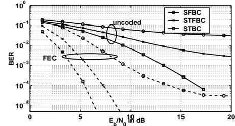
Fig. 11. BER of space-frequency block code (SFBC), space-time-frequency block code (STFBC) and space-time block code (STBC). Channel B,  $f_d T_{s,OFDM\_GI} = 0.01$ ,  $n_T = 4$ ,  $n_R = 1$ ,  $N_s = 1024$ , QPSK modulation, 3000 info bits per block.
