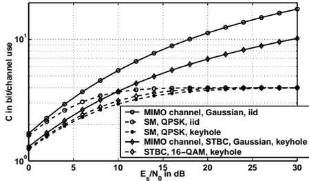
Fig. 4. Ergodic capacity for keyhole channel  $n_T = n_R = 2$ . Spatial multiplexing (SM) with QPSK, space-time block code (STBC) with 16-QAM.
