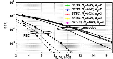
Fig. 12. BER of space-frequency block code (SFBC), space-time block code (STBC) and space-time-frequency block code (STFBC). Channel A,  $f_d T_{s,OFDM\_GI} = 0.01$ ,  $n_R = 1$ , BPSK modulation, 2000 info bits per block.
