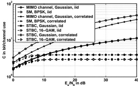
Fig. 3. Ergodic capacity for correlated MIMO channel  $n_T = n_R = 4$ . Spatial multiplexing (SM) with BPSK, space-time block code (STBC) with 16-QAM.
