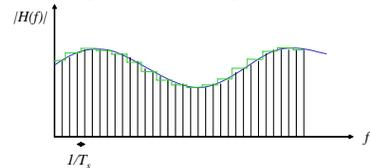
Fig. 5. Approximation of channel frequency response for orthogonal space-frequency block code.
