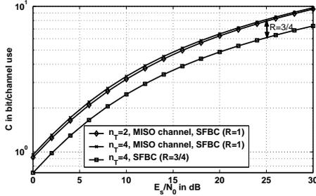
Fig. 6. Ergodic capacity for channel B and space-frequency block code (SFBC),  $n_R = 1$ ,  $N_s = 1024$ .
