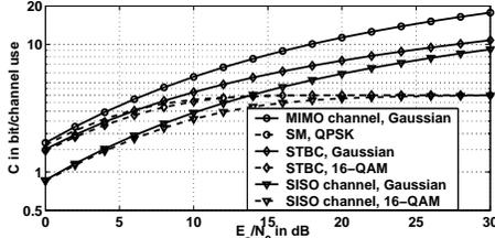
Fig. 2. Ergodic capacity for uncorrelated MIMO channel  $n_T = n_R = 2$ . Spatial multiplexing (SM) with QPSK, space-time block code (STBC) with 16-QAM.
