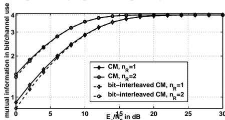
Fig. 7. Ergodic mutual information for space-time block code with coded modulation (CM) and bit-interleaved coded modulation (bit-interleaved CM),  $n_T = 2$ , 16-QAM with Gray mapping.
