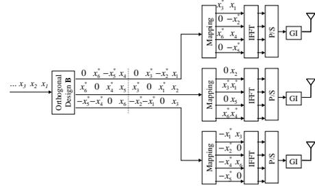
Fig. 8. Space-time-frequency block code in OFDM.  $N_s = 4$ ,  $n_T = 3$ .
