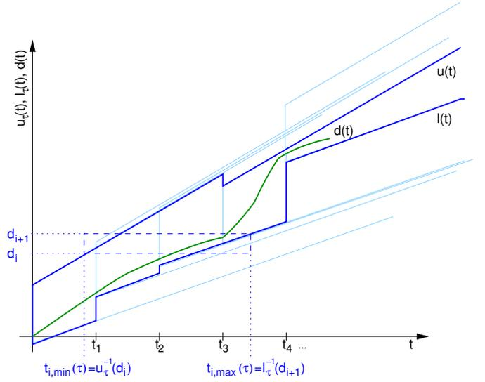
Fig. 2. Boundaries of Dynamic Movement Specification
