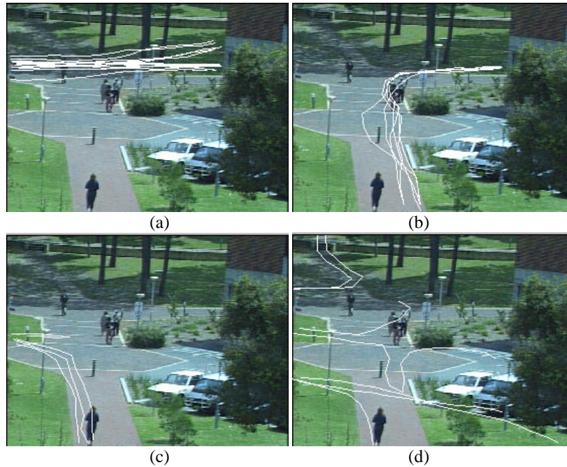
Figure 4. a-c) Classification of trajectories using route model. d) un-classified routes not recognised by the system.
