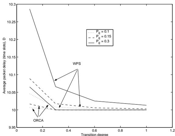
Fig. 4. Comparison between WFQ and ORCA in terms of long-term average packet delay.
