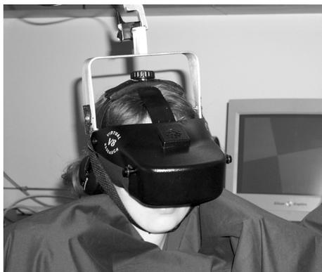
**Figure 2. Photograph of a subject wearing the system. Stops for the desired head positions are made from wood covered with foam and are under the black cloth in this picture.**
