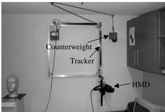
**Figure 1. Mechanical head tracker in its calibration jig. The tracker has four joints linked by rigid links and is anchored to the frame on the wall. Each joint has two independent rotational degrees of freedom. The weight of the tracker is counter-balanced by a weight and pulley system.**
