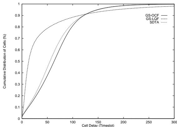
**Figure 1.** Cumulative distributions of cells under *i.i.d.* on-off traffic with a load of 80%.
