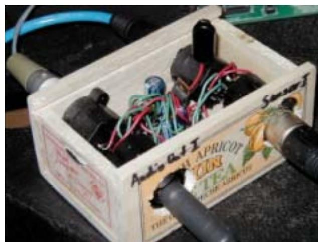
Figure 1. The TeaBox sensor-audio interface.
