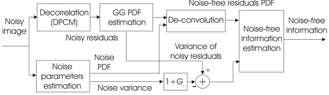
Figure 2: Flowchart of the proposed information-assessment procedure from a digital image.
