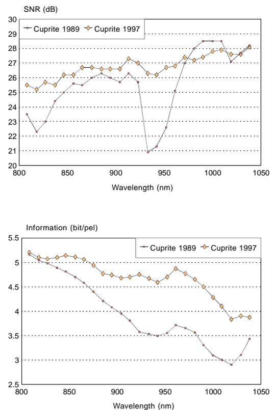
Figure 5: SNR and mutual information of 25 bands from the two AVIRIS sequences, varying with the wave-length.
