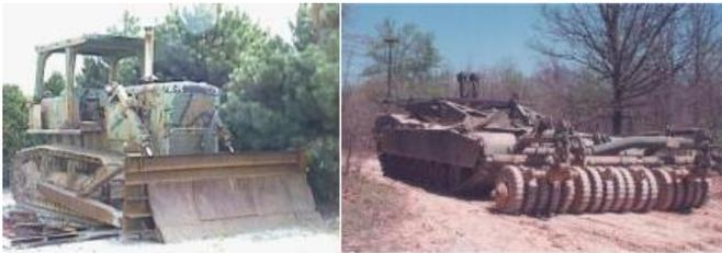
Fig. 10. Caterpillar D-7G and M1 PANTHER II built on a US Army M1 Tank base. Photos courtesy of UGV/S JPO.
