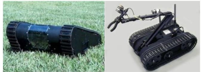
Fig. 7. Foster-Miller MATILDA (left) and Talon (right). MATILDA photo courtesy of UGV/S JPO. Talon photo courtesy of Foster-Miller.
