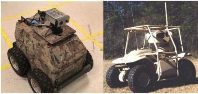
Fig. 8. iRobot ATRV-Jr shown here in camouflage (left). SARGE built on a Yamaha Breeze ATV base (right). SARGE photo courtesy of UGV/S JPO.
