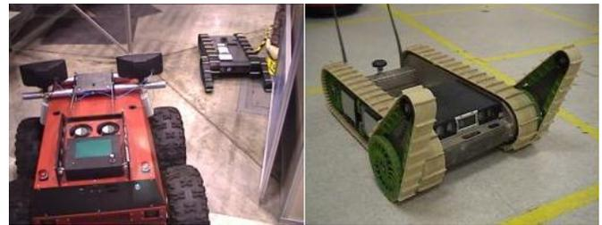
Fig. 6. iRobot Urban and ATRV (left). iRobot Packbot (right).
