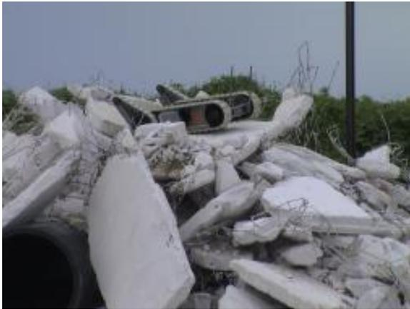
Fig. 2. An iRobot Packbot climbing a rubble pile used for USAR training.
