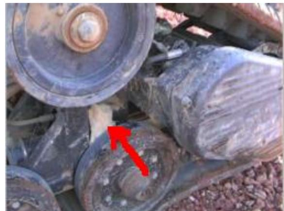
Fig. 12. Rock stuck in ARTS track mechanism. Photo taken from ARTS study.[20]
