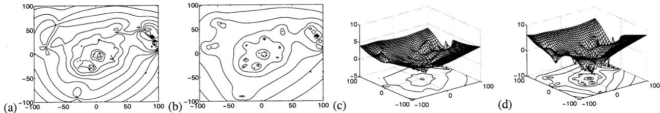
Fig. 5. Scene with a set of randomly placed landmarks. (a) Contour map of the log of the trace of the covariance map. (b) Contour map of the log of the determinant of the covariance map. (c) and (d) Surfaces of these two uncertainty functions. The localization algorithm does best close to two very close landmarks and does also well next to four landmarks a bit further apart.
