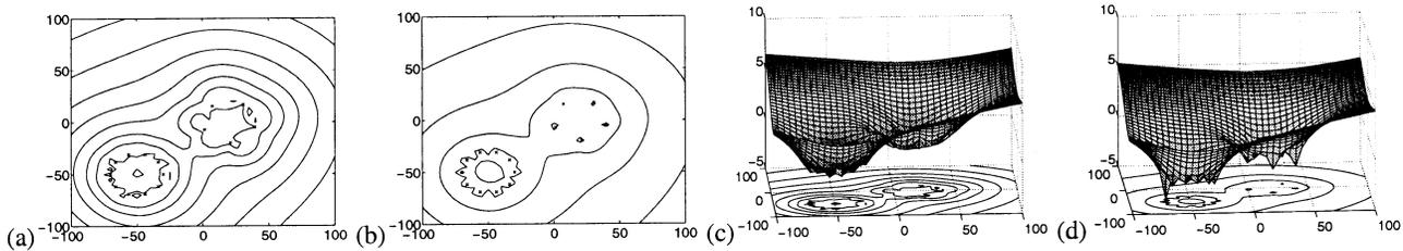
Fig. 4. Scene with two circles of landmarks with ten and five landmarks each, landmarks are marked with  $x$ 's. (a) Contour map of the log of the trace of the covariance map. (b) Contour map of the log of the determinant of the covariance map. (c) and (d) Surfaces of these two uncertainty functions. Best results obtained near the landmarks of the circle with more landmarks.
