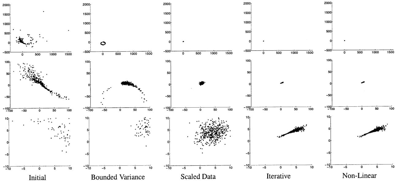
Fig. 3. For each of the five algorithms, we present the distribution of the results obtained from running it on 500 experiments. The correct answer is (4, 4) the landmarks lie within a circle of radius 100, and the measurement error is normally distributed with standard deviation of  $5^\circ$ . The results are plotted three times in different scales.
