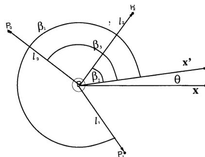
Fig. 1. Illustration of a planar mobile robot which detects three known landmarks in directions  $\beta_1$ ,  $\beta_2$ ,  $\beta_3$ . The goal is to find the robot's position and orientation in the plane.
