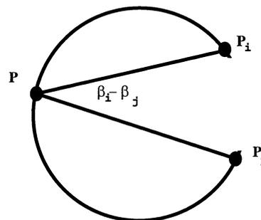
Fig. 2. Given two landmarks  $\mathbf{P}_i$  and  $\mathbf{P}_j$  whose bearing measurements are  $\beta_i$  and  $\beta_j$ , respectively. The possible robot positions lie on a circle illustrated in the figure.
