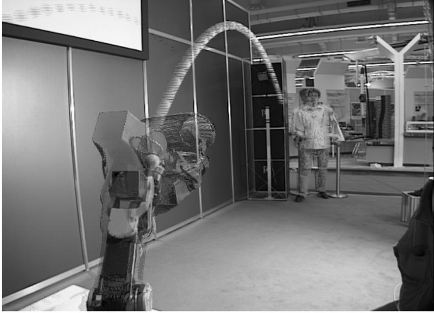
Figure 6: Example of a successful catch. The image shown is an overlay of a video sequence.
