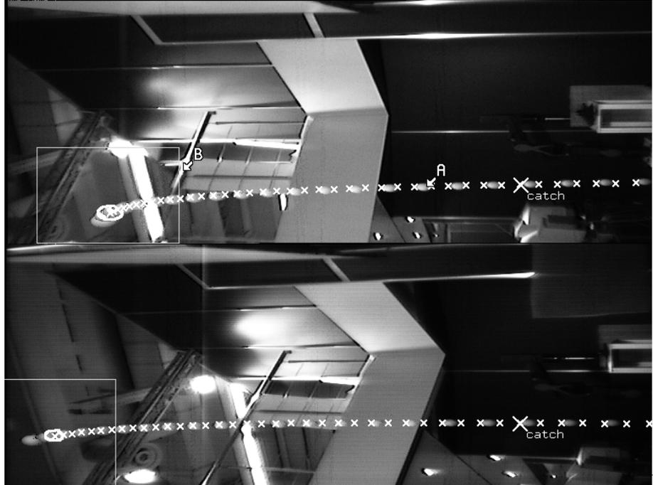
dictions as a function of time. One can observe the high accuracy ( $< 10\text{cm}$ ) achieved even for the early predictions, with the major error occurring in the direction of the throw (x-axis in the figure). Figure 8 shows the throw as seen by the cameras. Overlaid is a early prediction of the trajectory.
