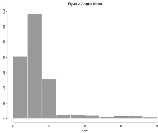
Figure 2: Histogram of the angular errors between the actual and recovered surface normals.
