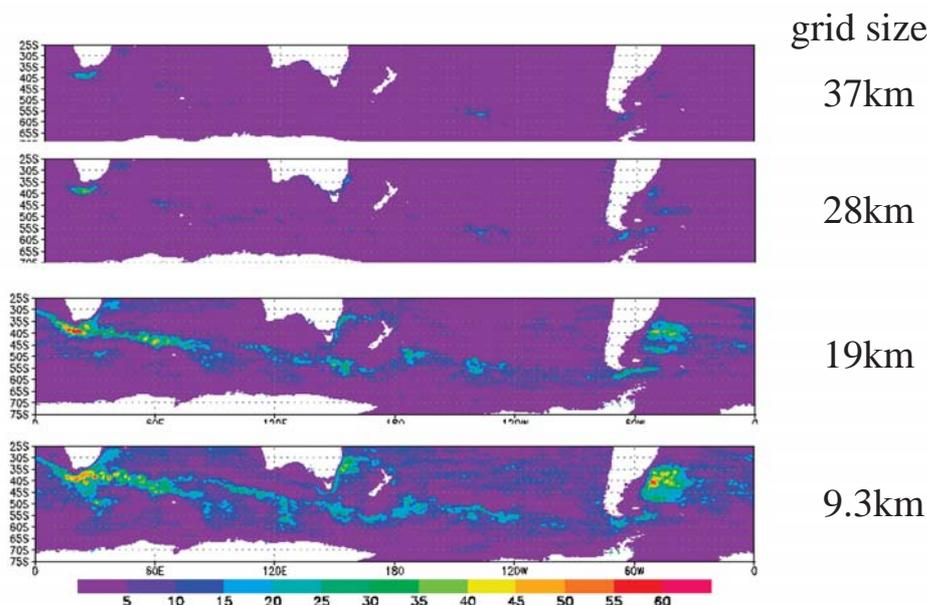
Fig. 6 Sea surface height anomaly variability (cm) calculated using from 9.3 to 37 km grid size. The time integration is carried out for 12 years and the last one year variability is shown.
