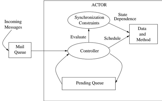
Fig. 8.4. An actor with local synchronization constraints.
