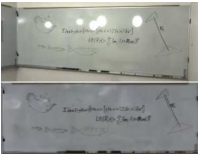
Figure 9: The top picture is a radiance image of a whiteboard, showing strong specular highlights. The bottom picture shows the diffuse albedo map of the whiteboard recovered from several images. Unlike the radiance image, the diffuse albedo map has a nearly uniform background, and is independent of the illumination.
