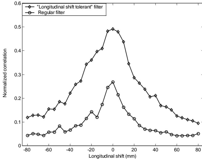
Figure 6. Value of the output peak versus longitudinal shift along the  $z$ -axis. Comparison between a filter made with focused images (“regular filter”) and a filter including defocused images (“longitudinal shift tolerant filter”).
