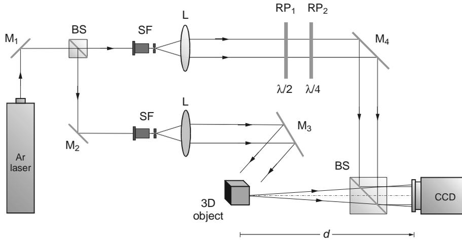
Figure 1. Experimental setup -M mirror, BS beamsplitter, SF spatial filter, L lens, RP retardation plate.
