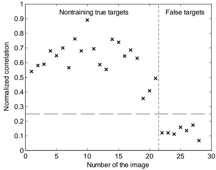
Figure 7. Correlation results obtained with various test objects. Filter made from 15 focused and defocused views based on one single hologram.
