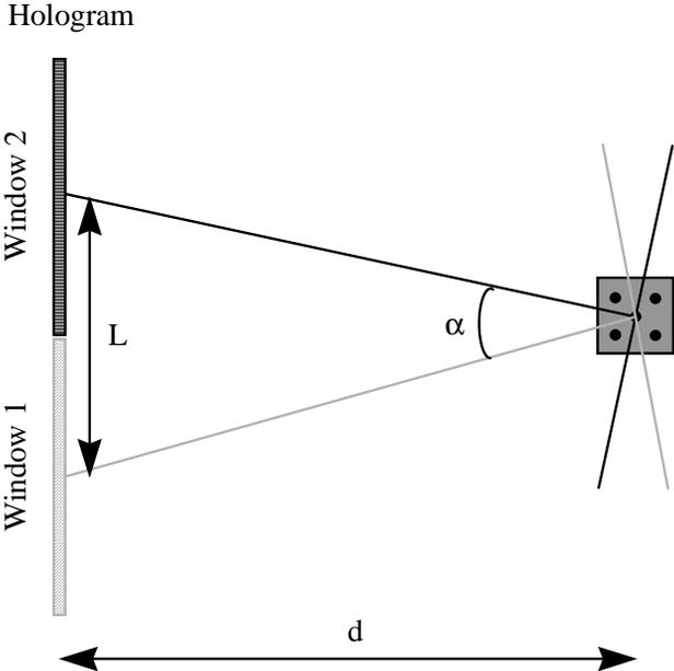
Figure 3. Shifting the reconstruction window inside the hologram results in changing the angle of view of the object.
