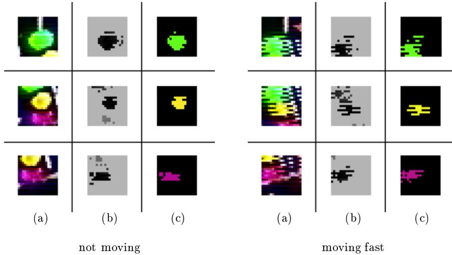
**Fig. 2.** Segmentation of colored dots in HSI space. Shown are (a) the original images, (b) the saturation/intensity masks, (c) and the segmented pixels, that have been selected using the hue distance to the model.
