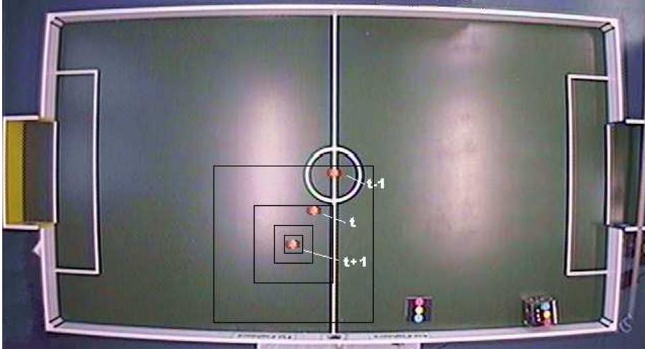
**Fig. 1.** A typical camera image, showing the field with shadows at the walls and reflections in the center. The linear ball prediction and a variable search window are shown too. The robots are marked with three colored dots.
