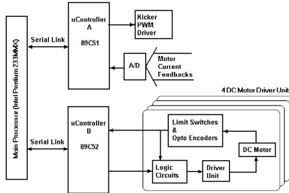
Fig. 4. Player robot hardware components interconnection diagram
