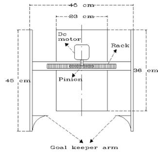
Fig. 3. Sliding arm movement
