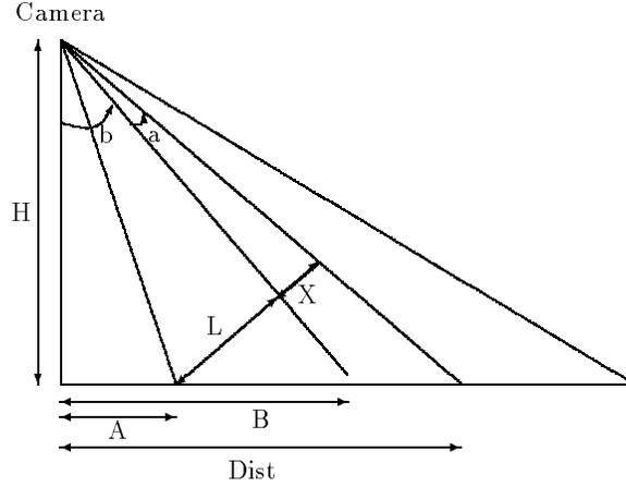
**Fig. 5.** Geometrical relations for finding object distance
