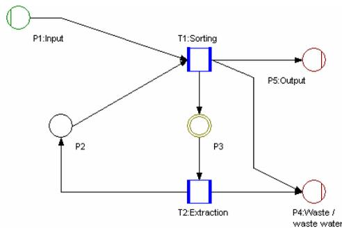
**Figure 1.** Simple material flow network (process water cycle)
